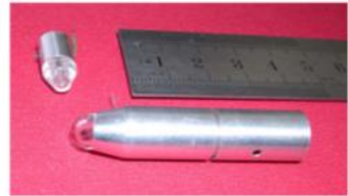
Fig.1: Early non ingestible wired devices with a 1/4" CCD used for testing the optics and the illumination
